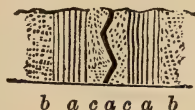
FIG. 298.—DYKES OF BASALT ( a a a ) TRAVERSING CHALK ( b ), WHICH NEAR THE DYKES IS CONVERTED INTO MARBLE ( c ), RATHLIN ISLAND, ANTRIM.
